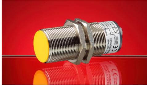
It's a rotation control device with the shape of a cylindrical threaded metallic sensor M30x1.5 inductive sensing featuring an activating distance between 4 and 6 mm on metallic material.
